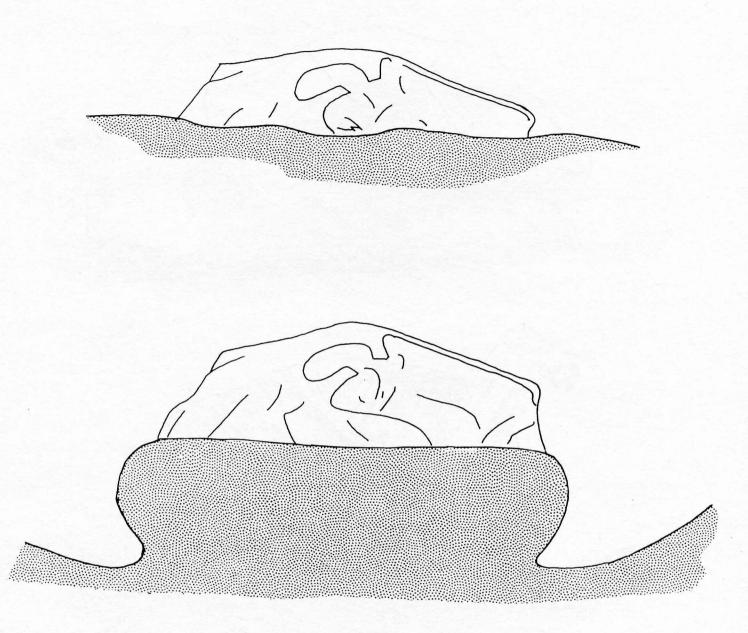
FIGURE 4-4. Top, specimen as discovered in the ground. Bottom, excavation work is done leaving ample matrix around the specimen and a generous undercut.
